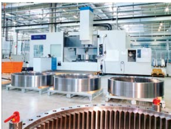
Berthiez maskin dreiesenter for dreining, boring, fresing.
