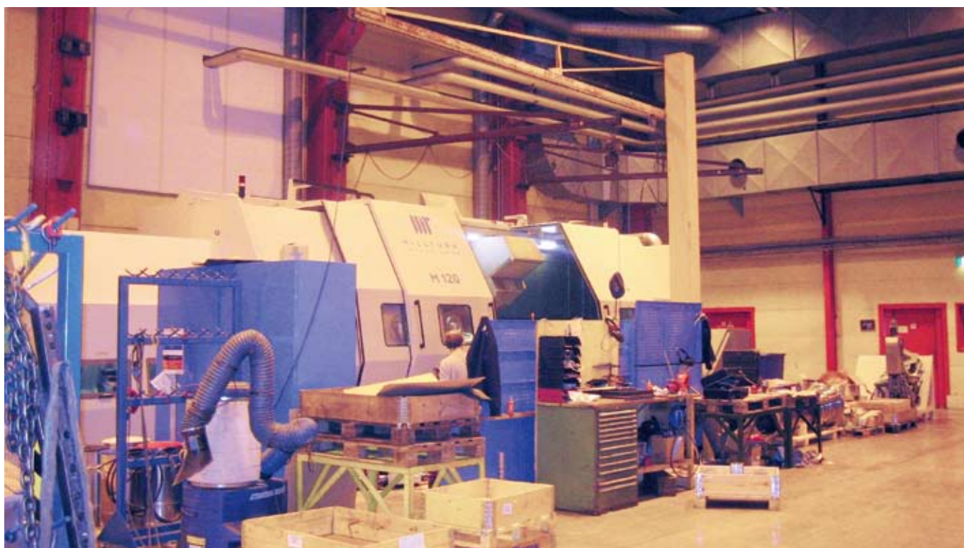
WFL komplettbearbeidings dreiesenter for boring, dreining, fresing, type M120, 2 stk. levert Frank Mohn Flatøy AS.
