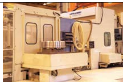
Mitsui Seiki horisontalt maskineringscenter type HS5-80, levert Aker Solutions Tranby
